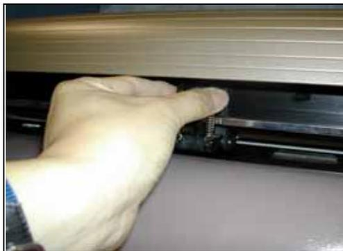
**Figure 2-15 Correct way to move pinch rollers**
